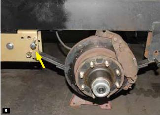
rear-axle spring sets connect to a patent-pending center section that isolates each axle, so the two springs are no longer connected by a central equalizer. The Liberty Rider is a complete system, meaning that the original suspension — including leaf springs, shackles, equalizers and shocks (if any) — are removed and discarded.
