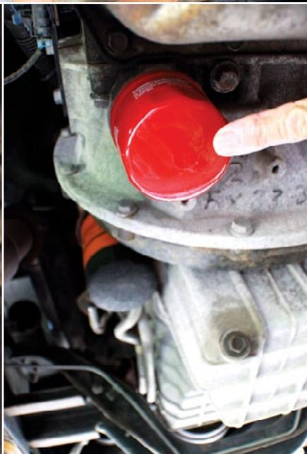
**Clockwise from top:** This is an example of the drain plug that comes standard on current-model transmissions. The red transmission oil filter is used mainly on Allison transmissions. The white engine oil filter shown here is mounted in a vertical position, making it practical to fill with oil before installation.
