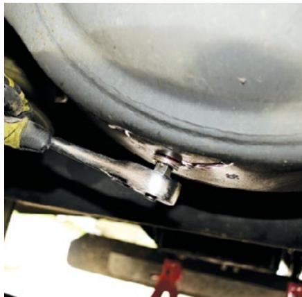
Removal of drain plug on rear differential can be accomplished by using a ratchet.
