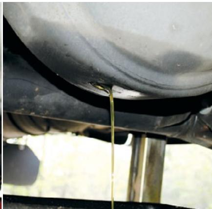
Make sure the oil from a third-member rear differential is completely drained into an oil catch basin.
