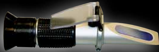
A refractometer is used to test the percentage of propylene glycol in the Aqua-Hot system's antifreeze.
