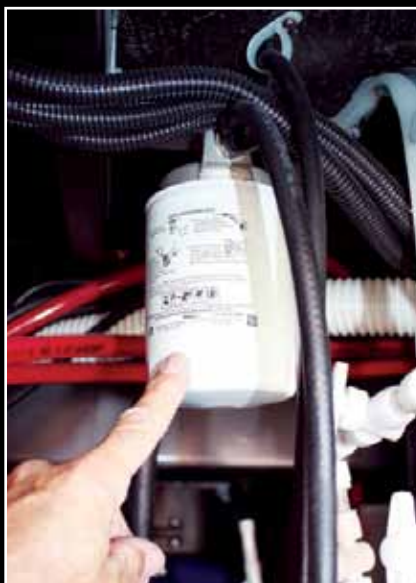
The Aqua-Hot fuel filter is commonly overlooked and must be changed annually.
