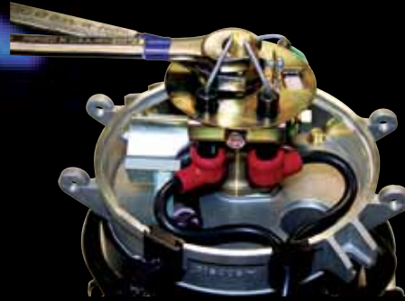
Removing the nozzle from the Aqua-Hot burner assembly requires the use of two wrenches, one on the backing nut and one on the nozzle.
