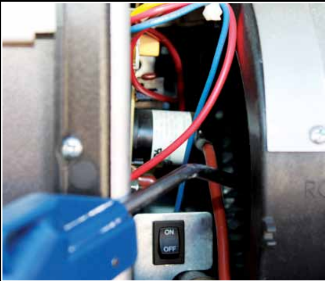
Accessing the Suburban furnace's blower wheel can be a challenge. However, it is important that area be cleaned on an annual basis using compressed air.
