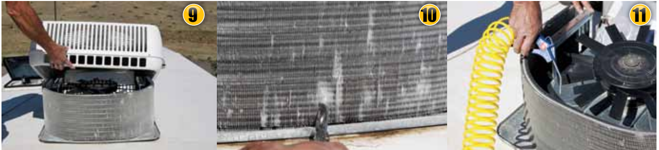
9) Annual A/C maintenance includes removing the shroud and inspecting condenser and wiring. 10) Check condenser for debris or bent fins. For optimum performance, straighten damaged fins using a thin tool. Use an evaporator comb if damage is extensive. 11) Clean condenser with low air pressure, taking care not to damage the delicate fins. A clean condenser makes the A/C more efficient.
