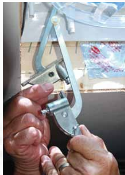
When installing the 6600R kit in an older Fan-Tastic Vent, the crank arm will need to be replaced. This will allow the vent to function properly when fully opening the lid.
